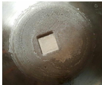
Fig. 2: The Ag- cube helps conducting heat between metals and fluid
