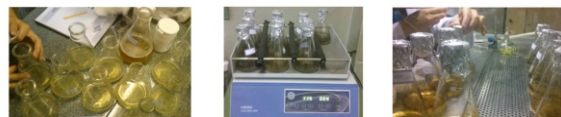
Fig. 1: The liquid culture medium before sterilization, the samples on a shaker, adding soil to culture medium; three different procedures (from left to right)
