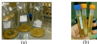
Fig.3: a) The produced biosurfactant , b) after centrifuge
