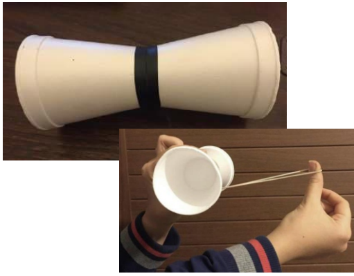
FIG.7: process of making a simple Magnus glider. By tracking a video of experiments with "tracker" program, the location was drawn (Fig. 8).
