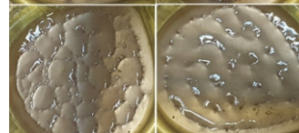
Electric Honeycomb Nazila Sharifi Farzanegan 1 High School Presented in PYPT 2016/ IYPT 2016 A vertically oriented steel needle over a horizontal metallic plate with some oil and constant high voltage between the needle and the plate will make a cell structure on the surface of the liquid.
