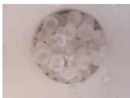
Fig 10: Salt particles inside the hole
