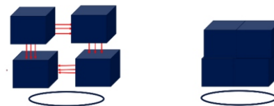
Fig 3 : Agglomeration making bigger particles
