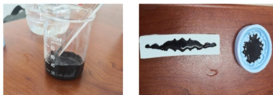
Fig. 2: Production and molding of KP based bioplastics
