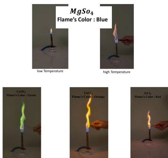
Fig. 4: Flame's color with different chemical substances
