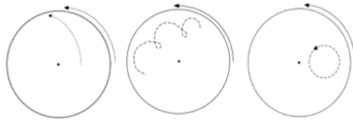
Fig. 4: (a) The ball expells from disc. (b) The ball makes loops (c) The ball runs on a circular orbit
