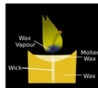
Fig. 2: A candle consists of a wax cylinder with a wick through the center. The flame melts a pool of wax at the top.
