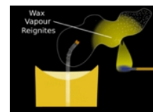
Fig. 5: The vapor is very flammable so you can relight it. Source: https://www.thenakedscientists.com/get-naked/experiments/jumping-flames
