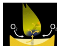
Fig. 3: The molten wax is drawn up the wick where it evaporates and then burns with the oxygen in the air. Source: https://www.thenakedscientists.com/get-naked/experiments/jumping-flames
