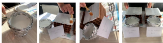
Fig.1: Preparation of the painted samples
