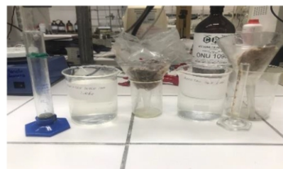
Fig. 7: Comparative test between double taboa filters with and without lemon at UFPE, Recife. Source: Authors (2022)
