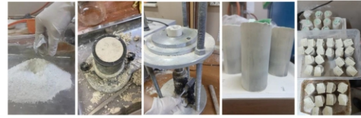
Fig.3: Preparation of Molds and Demoulding Process
