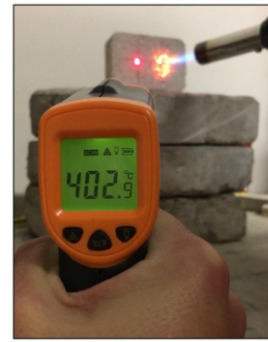
Fig. 8: Surface temperature readings were taken 3cm from the flame impact point (Picture: P.A. Huysamen)
