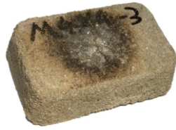
Fig. 6: Sample brick after being exposed to a butane torch flame for 2 minutes (Picture: P.A. Huysamen)
