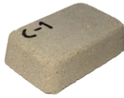
Fig. 3: Control sample brick C -1: eight volume portions sand and one volume portion cement (Picture: P.A. Huysamen)
