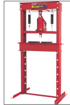
Fig. 5: A typical workshop hydraulic press Picture: (RP-20T, n.d)
