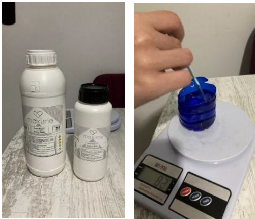
Fig.2: Mixing Epoxy Resin and Hardener
