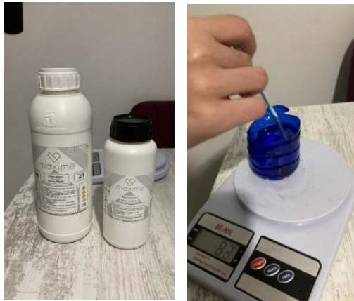
Fig.2: Mixing Epoxy Resin and Hardener
