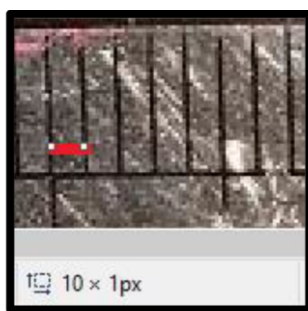
Fig. 5: The pixels of the line from one side to the other side of a millimeter of ruler drawn is shown in paint application
