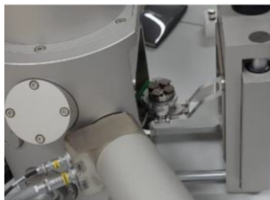
Fig. 13: Sample being inserted inside SEM (Author)
