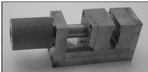
Fig.19 – The permanent magnet system used to measure Hall effect for the metal and semiconductor samples. The distance between two neodymium magnets can be easily changed obtaining magnetic field strength of about 1 T
