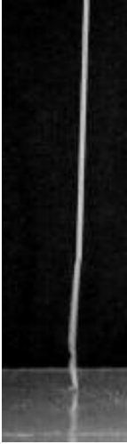
Figure 1: bending of spaghetti at the moment of impact
