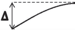
Figure 3: \Delta was measured while increasing the force applied to the end of the spaghetti
