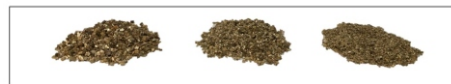
Fig. 1: (Left to Right) Grades of exfoliated vermiculite fine, super fine and micron (Picture: P.A. Huysamen)
