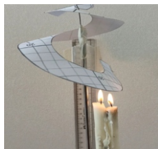
Fig.1: Paper spiral suspended above a candle
