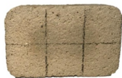
Fig. 7: Picture 7: Two crosses 3cm apart in the centre of the bottom brick face (Picture: P.A. Huysamen)
