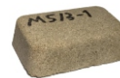
Fig.2: Sample brick M5/3 -1: five volume portions exfoliated micron grade vermiculite, three-volume portions sand and one volume portion cement (Picture: P.A. Huysamen)
