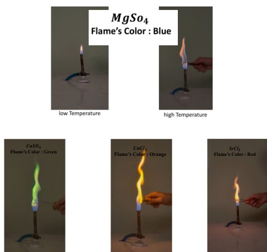
Fig. 4: Flame's color with different chemical substances
