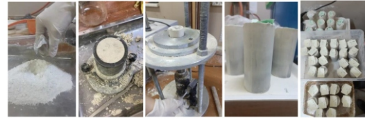
Fig.3: Preparation of Molds and Demoulding Process
