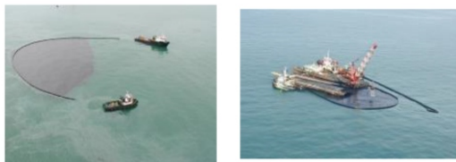
Fig. 2:U-shaped pulling of the barrier and the use of scrapers
