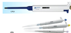
Fig. 2: Variable (A) and fixed (B) samplers
