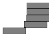
Fig. 6: The second disc doesn't move a lot because of the high number of the discs
