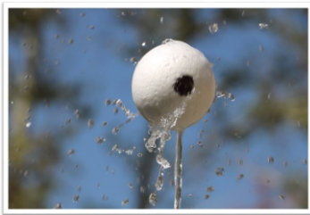
Fig. 1: Rotation of a Styrofoam disk on a water jet
